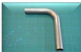
SUS304丸管材 42.7 × t1.5 × R80 SUS304 round pipe
