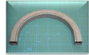
STKR角管材 30 \times 30 \times t1.2 \times Ri140 STKR square pipe
