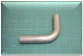
STKM丸管材 34.0 \times t1.6 \times R50 STKM round pipe
