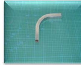
SUS304角管材 22×22×t1.2×Ri80 SUS304 square pipe
