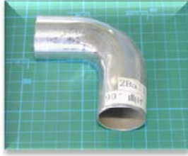
SUS304丸管材 38.1×t1.5×R40 SUS304 round pipe
