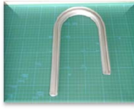
アルミ合金60系異型材 □23 × 20 × t1.0 × Ri62 Aluminum alloy(60 series)
