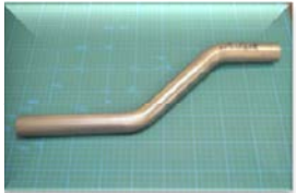
チタン(2種)丸管材 35.0 × t1.0 × R60 Titanium round pipe
