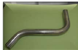
SUS304丸管材 65.0 × t1.5 × R130 SUS304 round pipe
