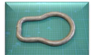
SUS304丸管材 22.0 × t1.5 × R30・75 SUS304 round pipe
