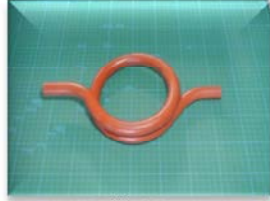
STB丸管材 21.7 × t4.0 × R70 STB round pipe
