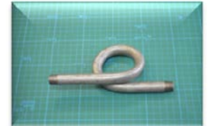
SUS316丸管材 17.3 × t2.0 SUS316 round pipe
