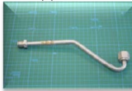
アルミ合金丸管材 9.53 \times t1.0 \times R13 Aluminum alloy(60 series) round pipe
