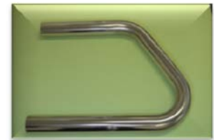
SUS304丸管材 48.6 × t2.0 × R90 SUS304 round pipe
