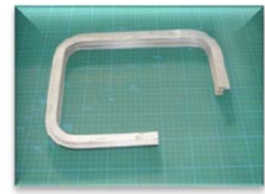
アルミ合金60系異型材 Z25 × 22.5 × Ri30 Aluminum alloy(60 series)
