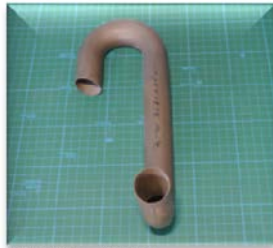
真鍮丸管材 31.8 × t0.6 × R 40 Brass round pipe
