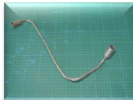
STKM丸管材 8.0 × t1.0 × R25 STKM round pipe
