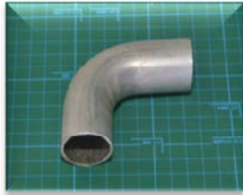
アルミ合金60系丸管材 31.8 × t1.5 × R32 Aluminum alloy(60 series) round pipe
