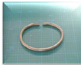
真鍮丸管材 10.0 × t1.5 × 複合R Brass round pipe
