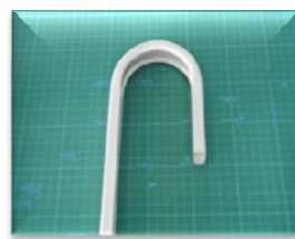
アルミ合金60系異型材 □25 × 13 × t1.0 × Ri40 Aluminum alloy(60 series)
