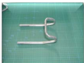
STKM丸管材 12.0 × t1.6 × R25 STKM round pipe
