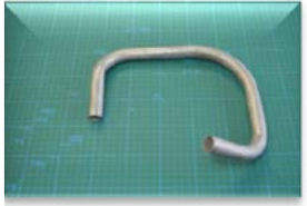
アルミ合金60系丸管材 22.0 \times t1.0 \times R50 \cdot 100 Aluminum alloy(60 series) round pipe
