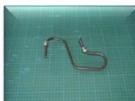
STKM丸管材 8.0 × t1.0 × R25 STKM round pipe
