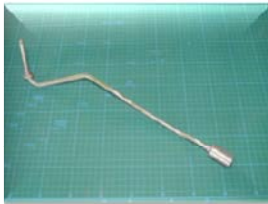
STKM丸管材 8.0 × t1.0 × R25 STKM round pipe
