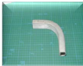
アルミ合金60系異型管材 D35 × 27 × t3.0 × Ri50 Aluminum alloy(60 series)
