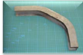
SS異型材 C40 \times 40 \times t2.3 \times Ro100 SS
