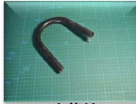
STKM丸管材 15.9 × t1.0 × R60 STKM round pipe
