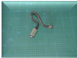
STKM丸管材 10.0 × t1.0 × R20 STKM round pipe
