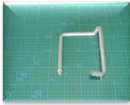
アルミ合金丸管材 12.7 × t1.0 × R12.7 Aluminum alloy(60 series) round pipe
