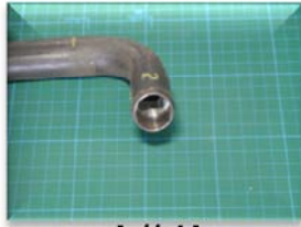
STPG丸管材 34.0 × t3.4 × R55 STPG round pipe
