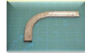
STKR角管材 40 \times 20 \times t1.6 \times Ri120 STKR square pipe
