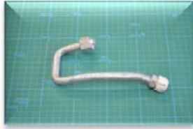
アルミ合金丸管材 12.7 \times t1.0 \times R15 Aluminum alloy(60 series) round pipe
